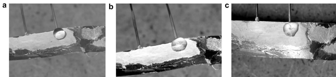
Fig. 1. Images of drops deposited on the unheated strip coated with a PAN nanomat. (a) immediately after deposition; (b) 10 min after deposition; (c) 17 min after deposition.
